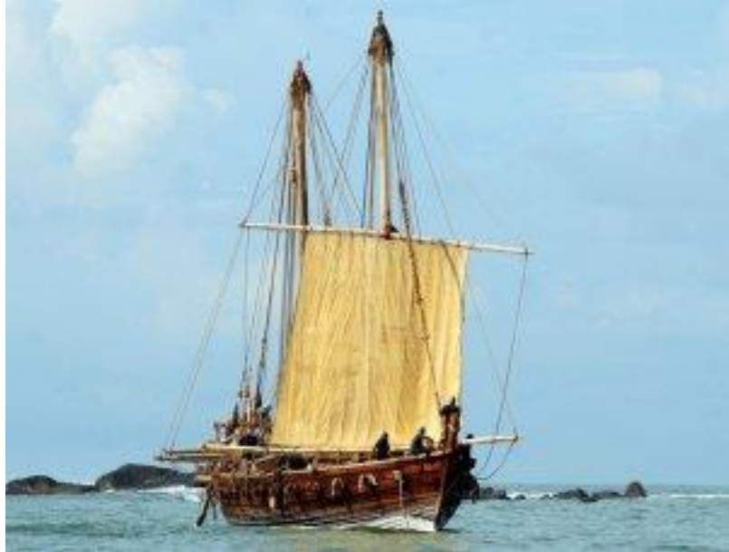
Arab dhows with hand-sewn, rather than nailed, planking were the staples of the intra-Indian Ocean trade before the arrival of Europeans in the region.
